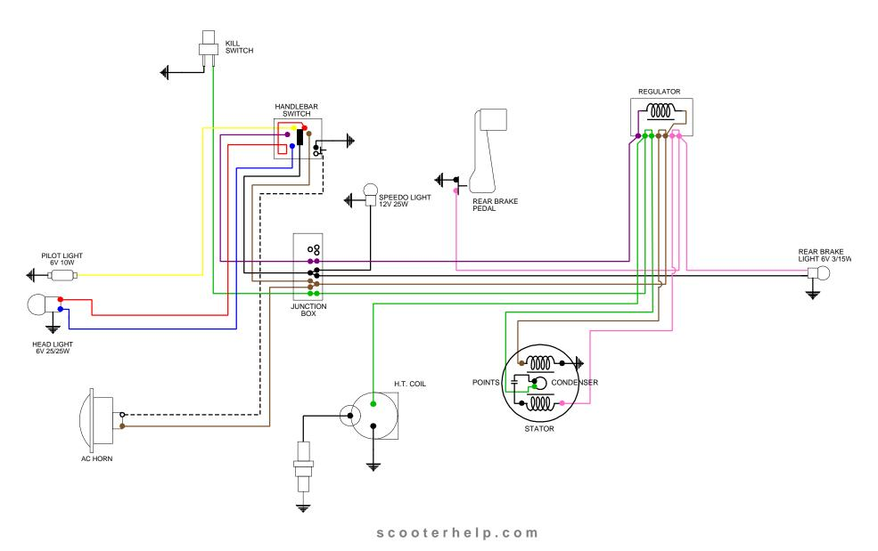
LAMBRETTA Li125 & Li150 Series 2 with 4 pole stator plate without battery
