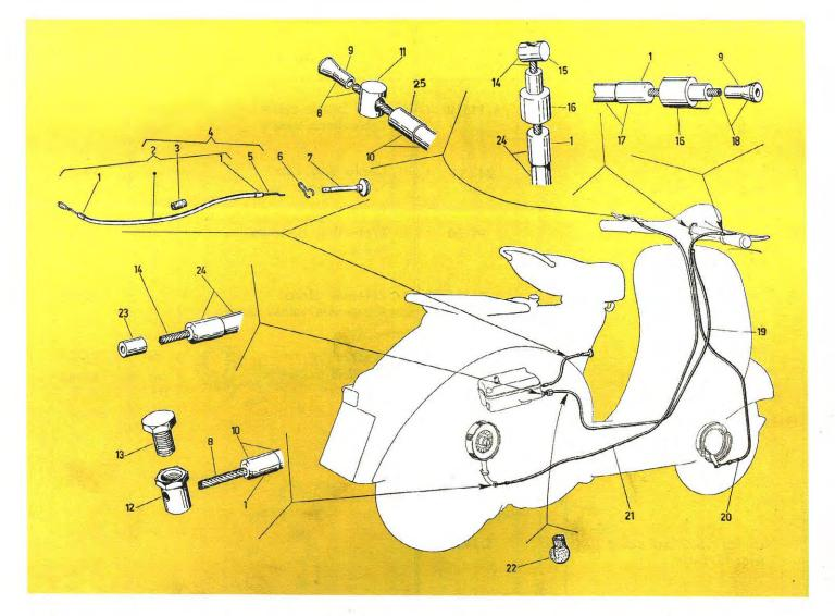
T. XVI Transmissions: Throttle - Clutch - Front brake
